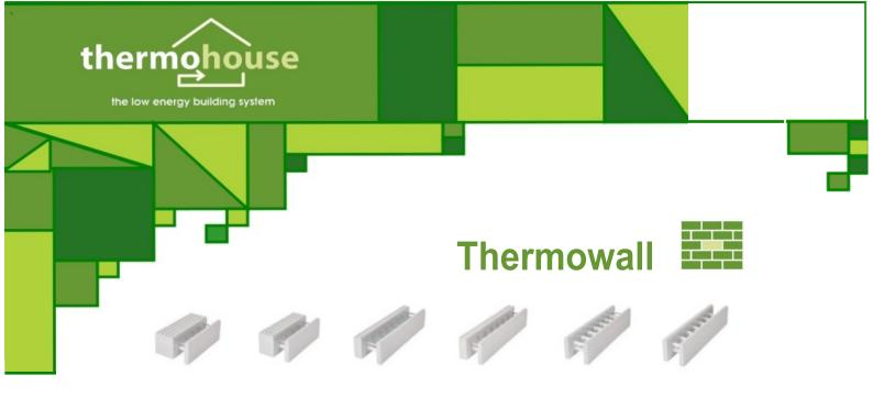
The Thermowall elements, made of expanded polystyrene (EPS), are applied as the formwork for plain or reinforced concrete walls cast in-situ. The Thermowall elements comprise of two leaves of EPS, which are connected by steel inserts to resist the pressure of the concrete during filling and vibrating. The upper and lower surfaces of the shuttering leaves are tongue and groove to place the elements together.
